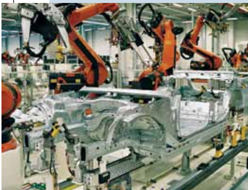
Spot-welding robots at the BMW plant in Leipzig, Germany.
